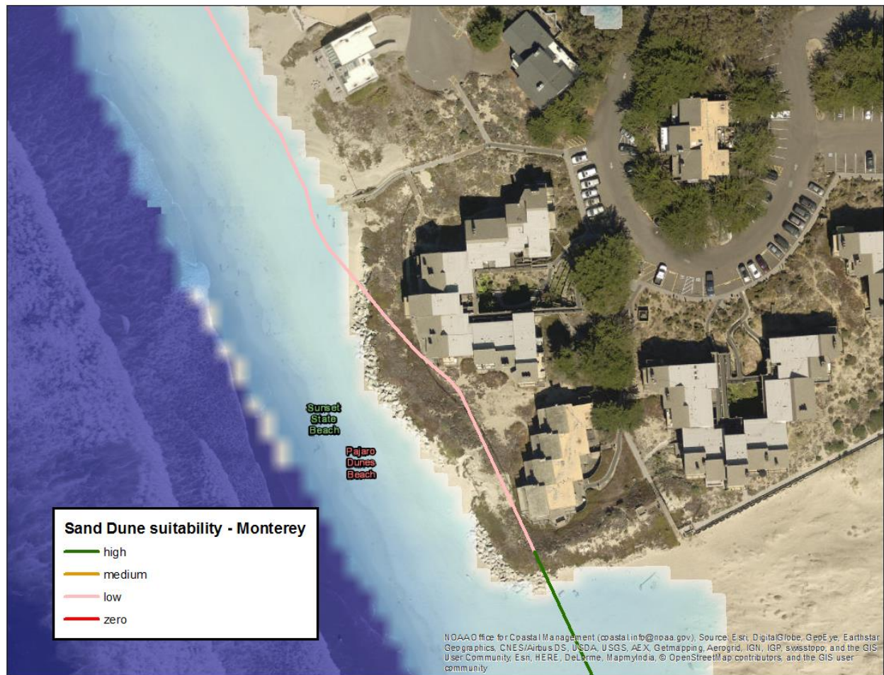
Figure E-2. Suitability for sand dune natural infrastructure measures up coast of the Pajaro river mouth in Santa Cruz County. The blue shading indicates the inundation extent with six feet of sea level rise.
