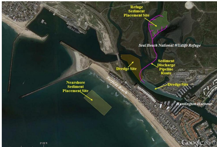
Figure F-4: Pipeline route from dredge site to augmentation site at the Refuge. The Nearshore Sediment Placement site was used in the larger dredging project and not the Seal Beach project.
